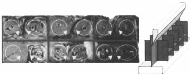
Figure 6: Vortex flow in a FELIX16 film when the air convection is conducted by a glass plate array (shown schematically at the right). The position of the plates is marked by horizontal and vertical lines. The flow field in the film is visible by advected \text{SmC}^* domain walls. A arrows indicate the reorientation sense of the vortices.
